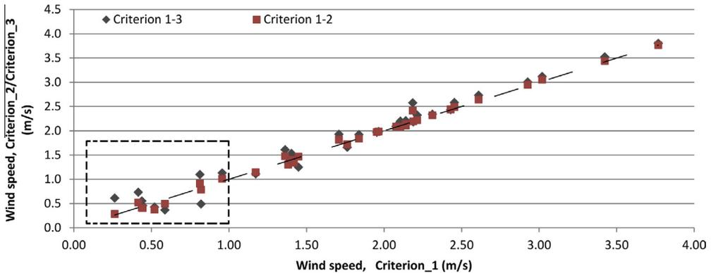
**Fig. 7.** Comparing results among three groups of wind data from the simulations with different iterative convergence criteria. Larger variance in the low wind speed area indicates that the simulation with the convergence criterion 3 is not sufficient in this case study.
