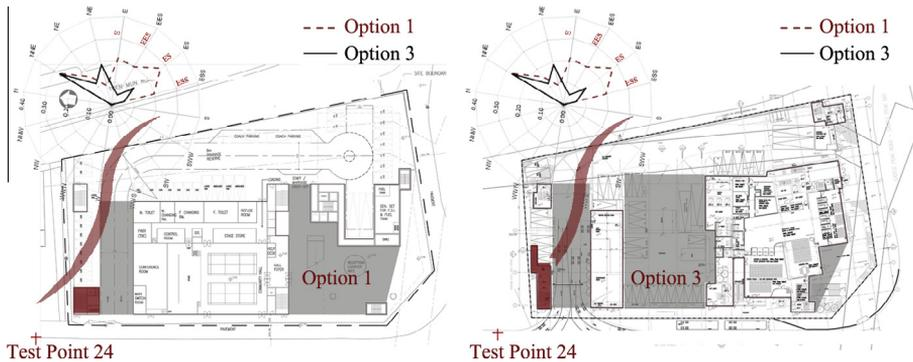
**Fig. 10.** Wind velocity ratios polar at the test point 24. The ground floor plan are presented together to illustrate how identify the part of the proposed building in option 3 that could block the incoming airflow.
